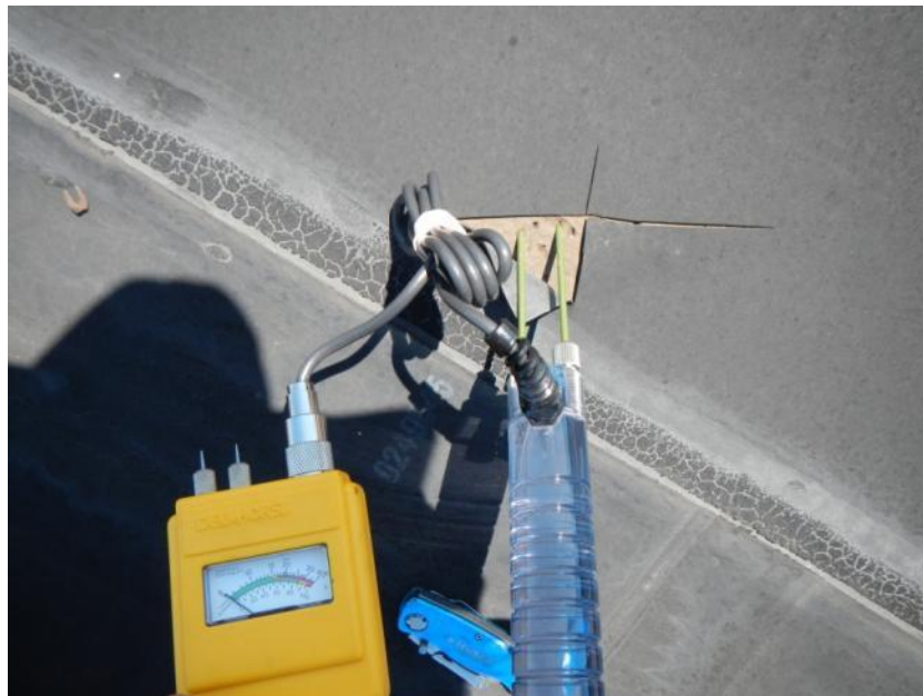
Opening Photograph 3 – Moisture meter reading using the 6" long probes.
