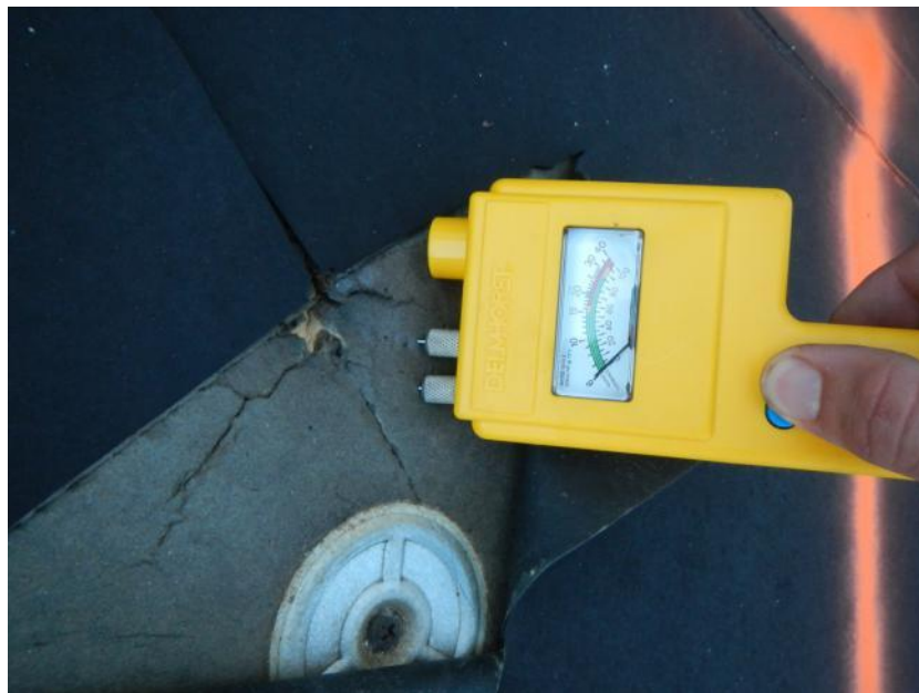
Opening Photograph 1 – The Delmhorst moisture meter showing a reading of no moisture.
