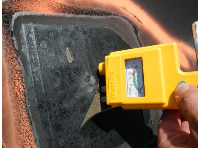
Opening Photograph 2 – Moisture meter reading no moisture content at this patch.
