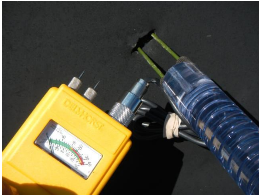
Opening Photograph 4 – Moisture meter reading using the 6" long probes in an existing membrane hole.
